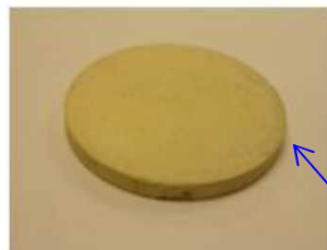
50 wt% AgI/50 wt% Glass, 500°C for 3 hr
