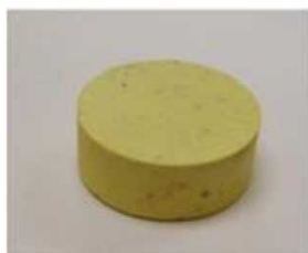
50 wt% AgI/50 wt% Glass 500°C for 3 hr
