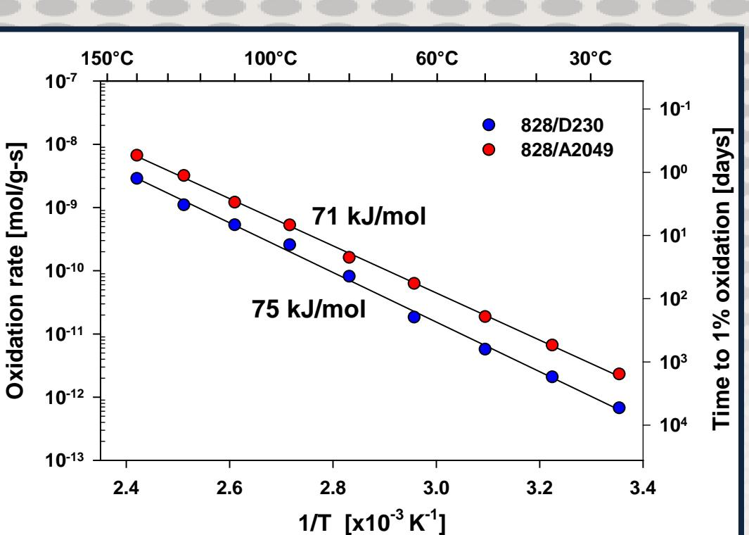
Oxidation rates are experimentally determined and available for many polymers including thermosets. Data provide consumed oxygen under non-DLO conditions. SNL has led this research activity.
