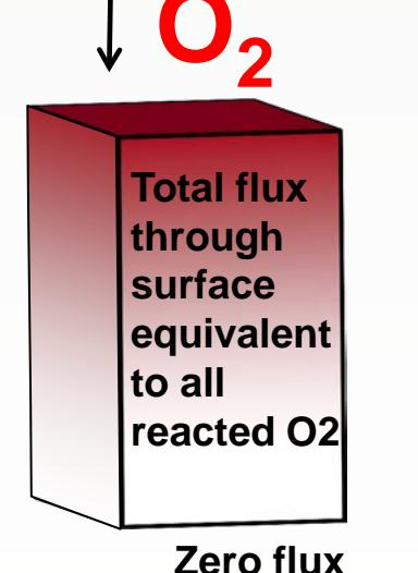
Prediction of oxygen flux and oxidation rate with respect to depth into an EPDM material for total material oxidation reactivity. The total flux can be analytically expressed:
