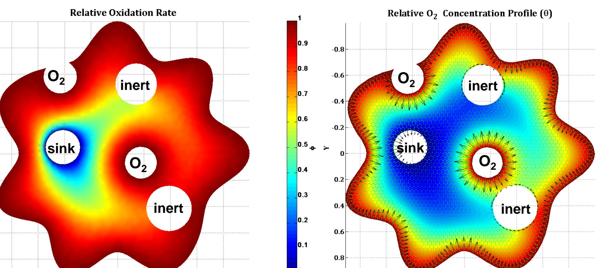
Model evaluation with multiple boundary conditions. Example of irregular domain, surface O<sub>2</sub> exposure, with internal inert voids, additional O<sub>2</sub> source, and an O<sub>2</sub> sink.
