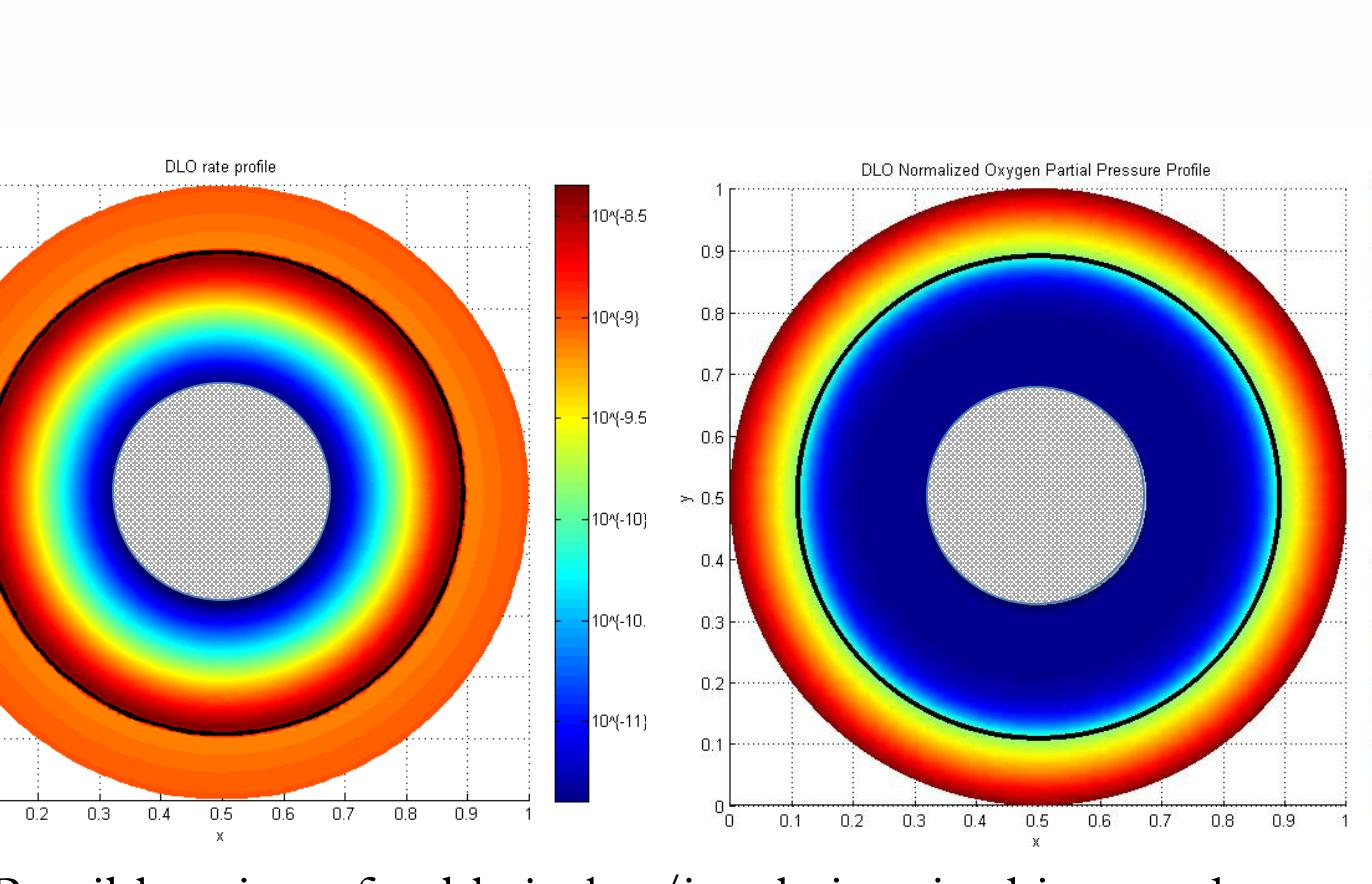
Possible aging of cable jacket/insulation, in this case the inner insulation has higher oxidation sensitivity and is DLO affected under accelerated aging conditions.
