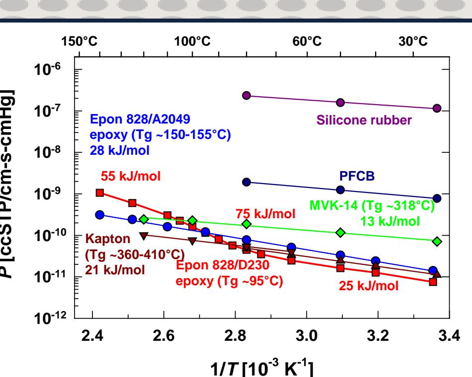
Oxygen permeability is obtained from flux measurements through thin films. O<sub>2</sub> diffusion and solubility are available via Fickian diffusion fits.
