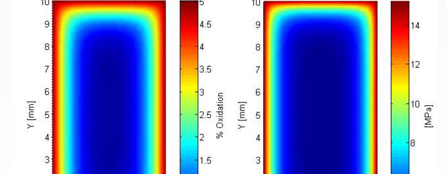
Prediction of DLO for cross-section of aged Neoprene at 125°C with changes in mechanical properties (oxidation level – modulus correlation from Modulus profiling).
