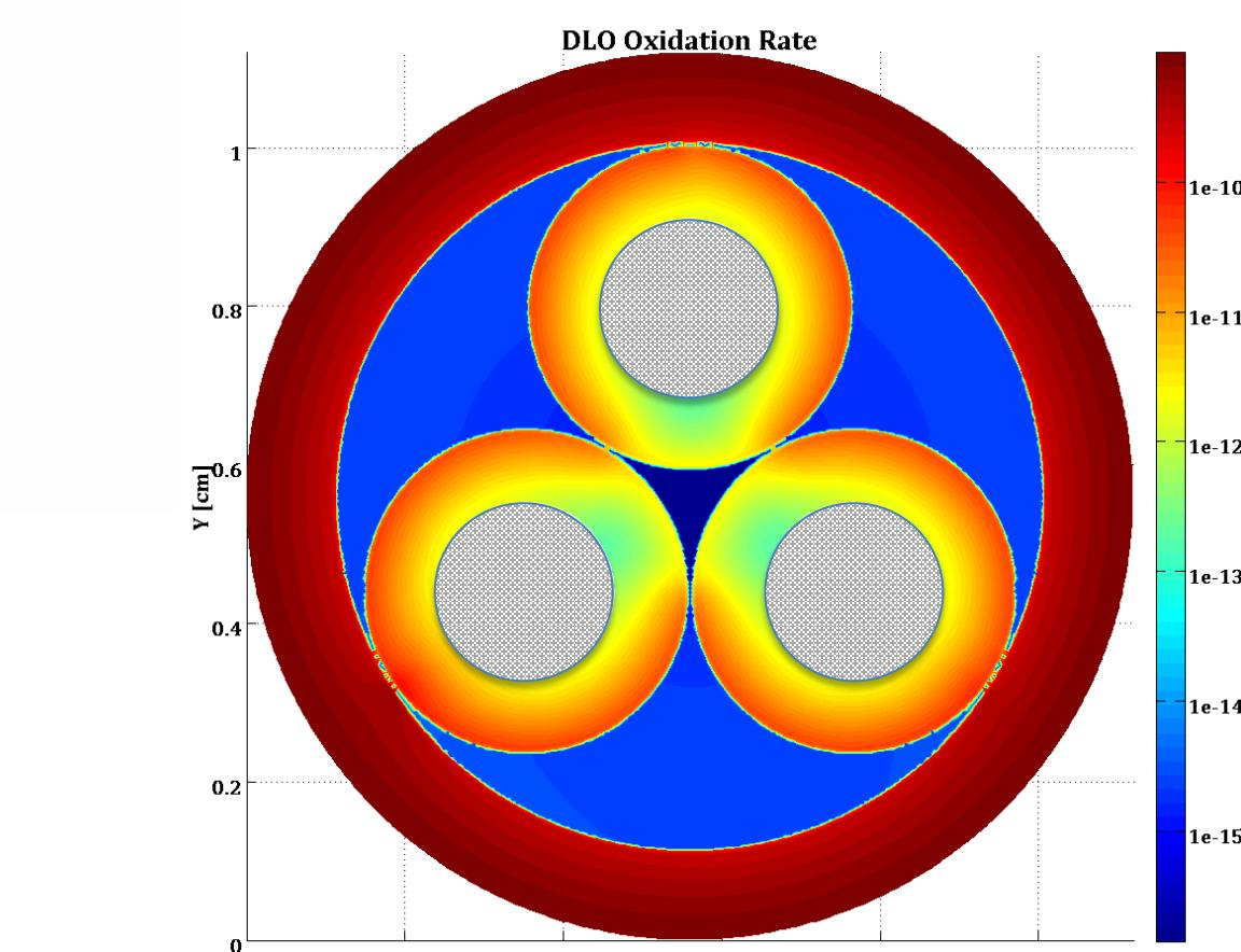
Potential aging in cable assembly. Weak gradient in jacket, DLO through insulation and restricted O<sub>2</sub> access in cable center
