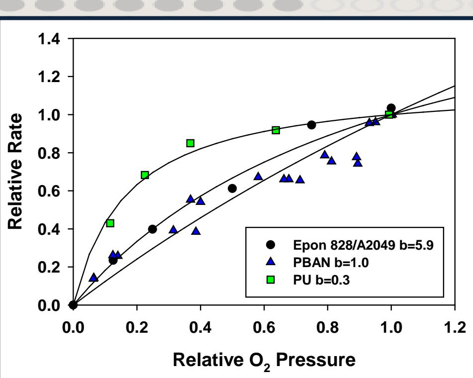
Oxygen rate dependence on local concentration, referenced to surface, is part of the mechanistic description and available from special rate experiments as well as DLO analysis.
