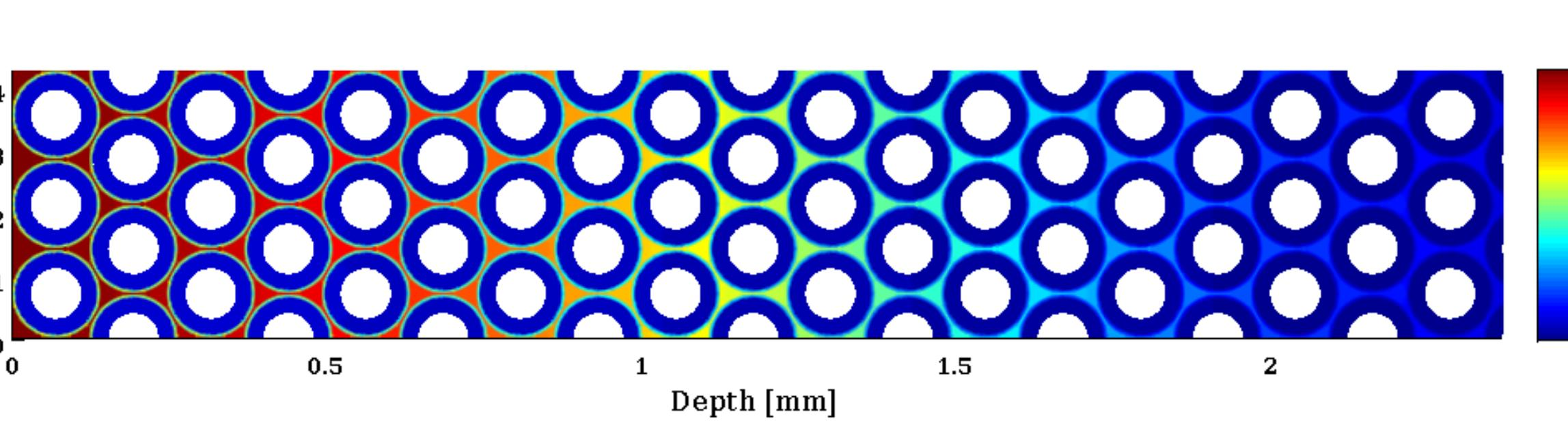
Spatially resolved oxidation rates for epoxy resin matrix and coated inert material assembly; two polymers with boundaries and complex permeation process; coating has a lower oxidation rate than matrix.
