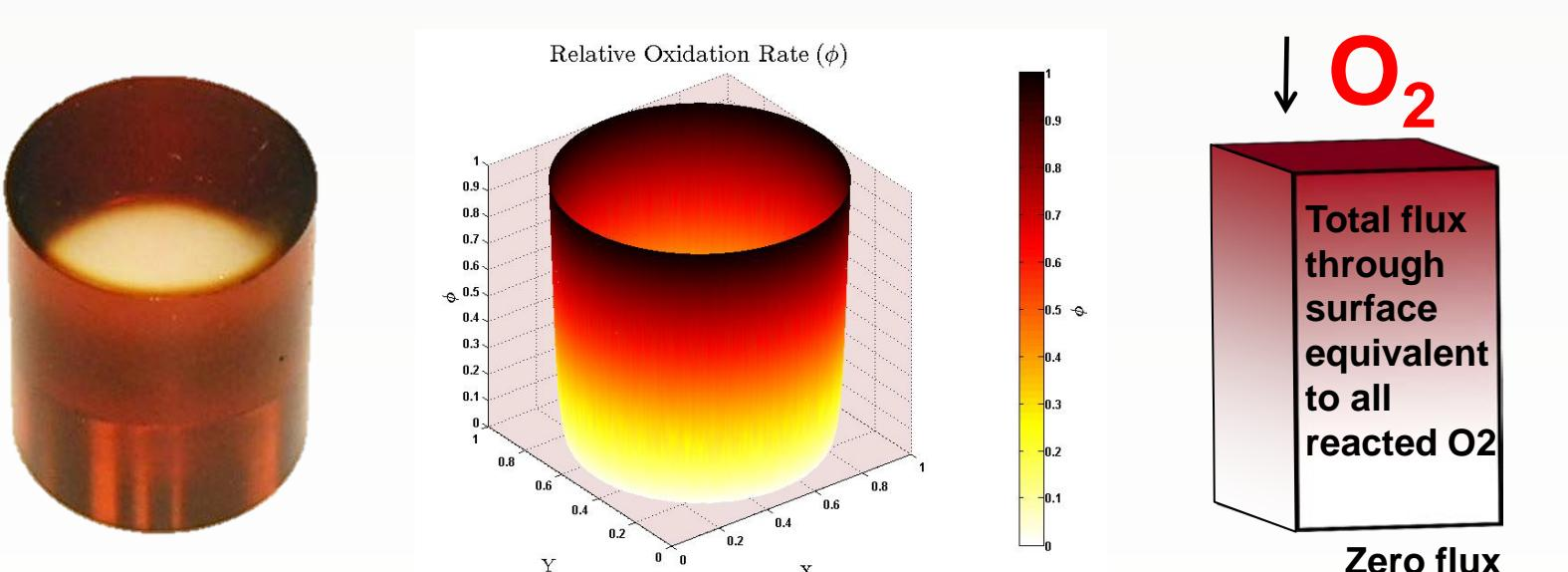
Actual degradation and model of an epoxy material where severe oxidation is limited to surface layer.
