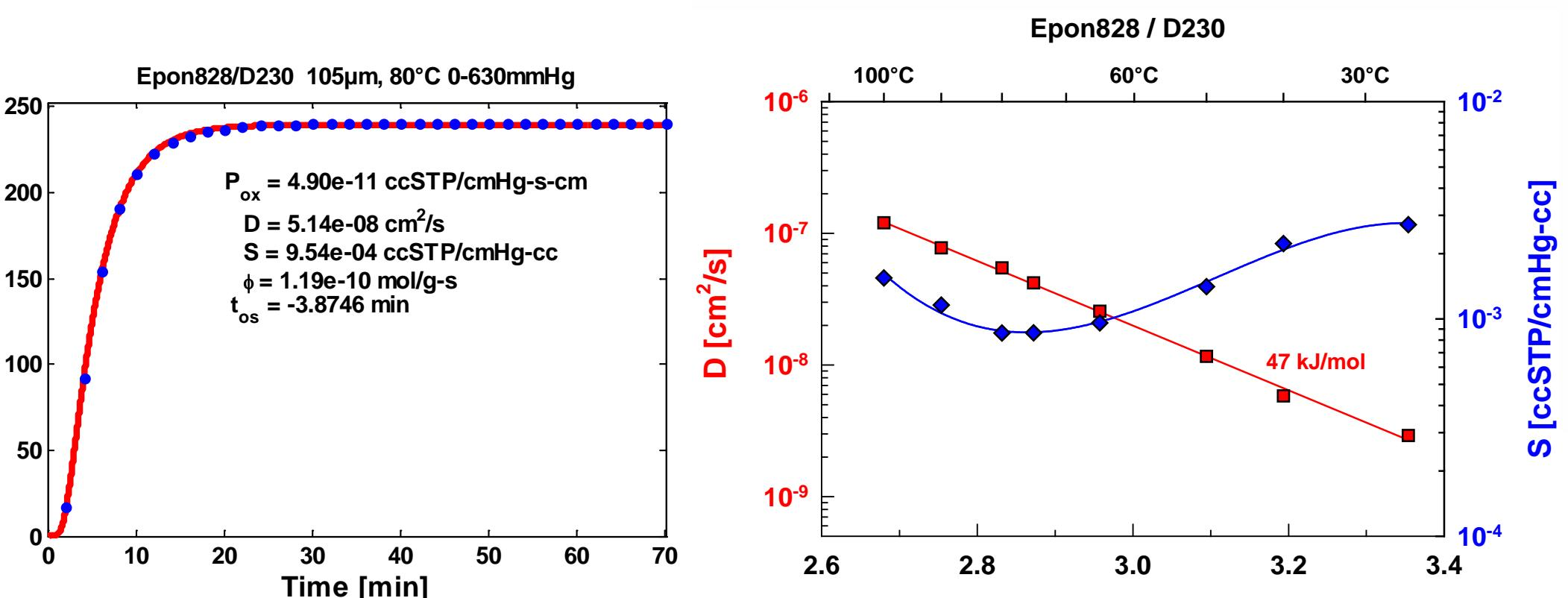
O<sub>2</sub> time – permeation flux measurements can be fitted with 1D film transport solution to extract permeability, diffusivity and solubility.
