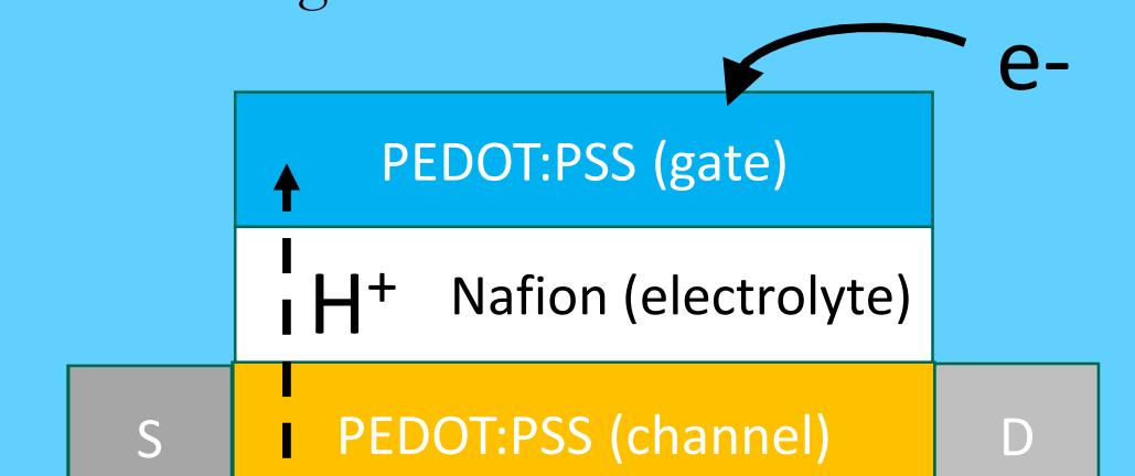
PEDOT:PSS is a redox-active polymer blend that undergoes a charge compensation reaction after proton insertion that generates hole carriers.
