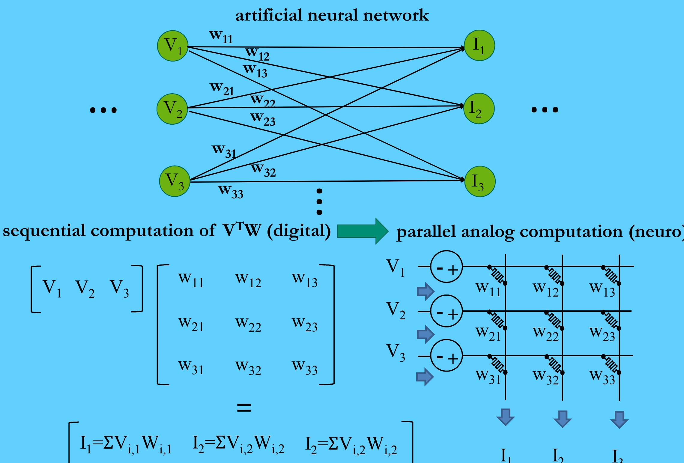
Resistive random access memory (RRAM) that is proposed for neuromorphic computers suffers from large voltages and currents that prevent scaling to large arrays.
