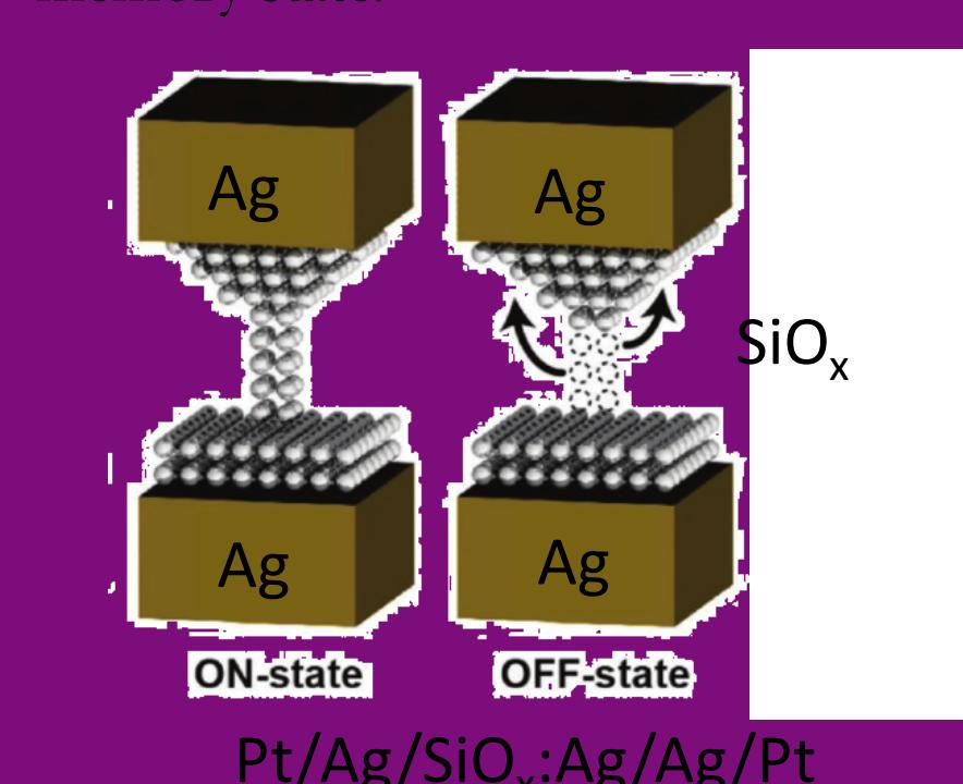
Once a small voltage threshold ( $\pm 400$  mV) is reached, the memristor turns to the ON state allowing the redox transistor to be programmed. A large ON/OFF ratio ensures long retention times. A fast filament dissolution time (150 ns) can support fast redox transistor programming times.
