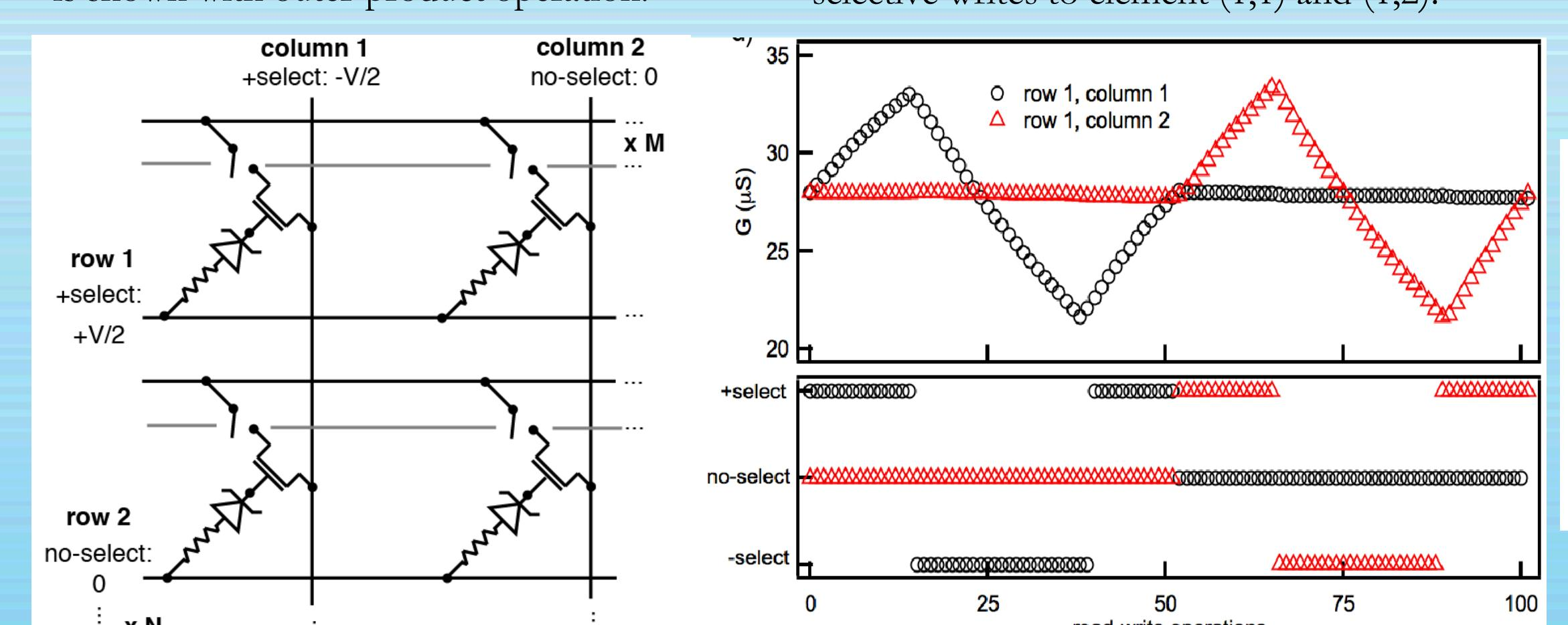
**Prototype IFG crossbar array** ( $1 \times 2$ ) with selective writes to element (1,1) and (1,2).
