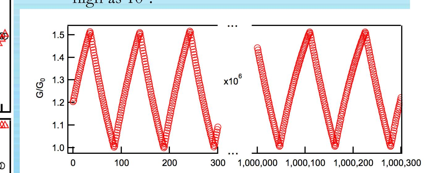
**Future work:** faster switching speeds  $> 1$  MHz, endurance  $10^{13}$ , and CMOS integration must be demonstrated.
