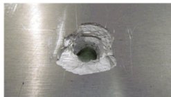
Damage level 5: Through hole
