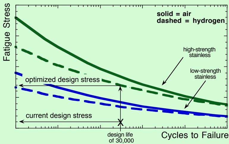
*This figure shows schematically the anticipated effects of hydrogen on fatigue and the performance improvement that can be realized by using high-strength austenitic stainless steels*
