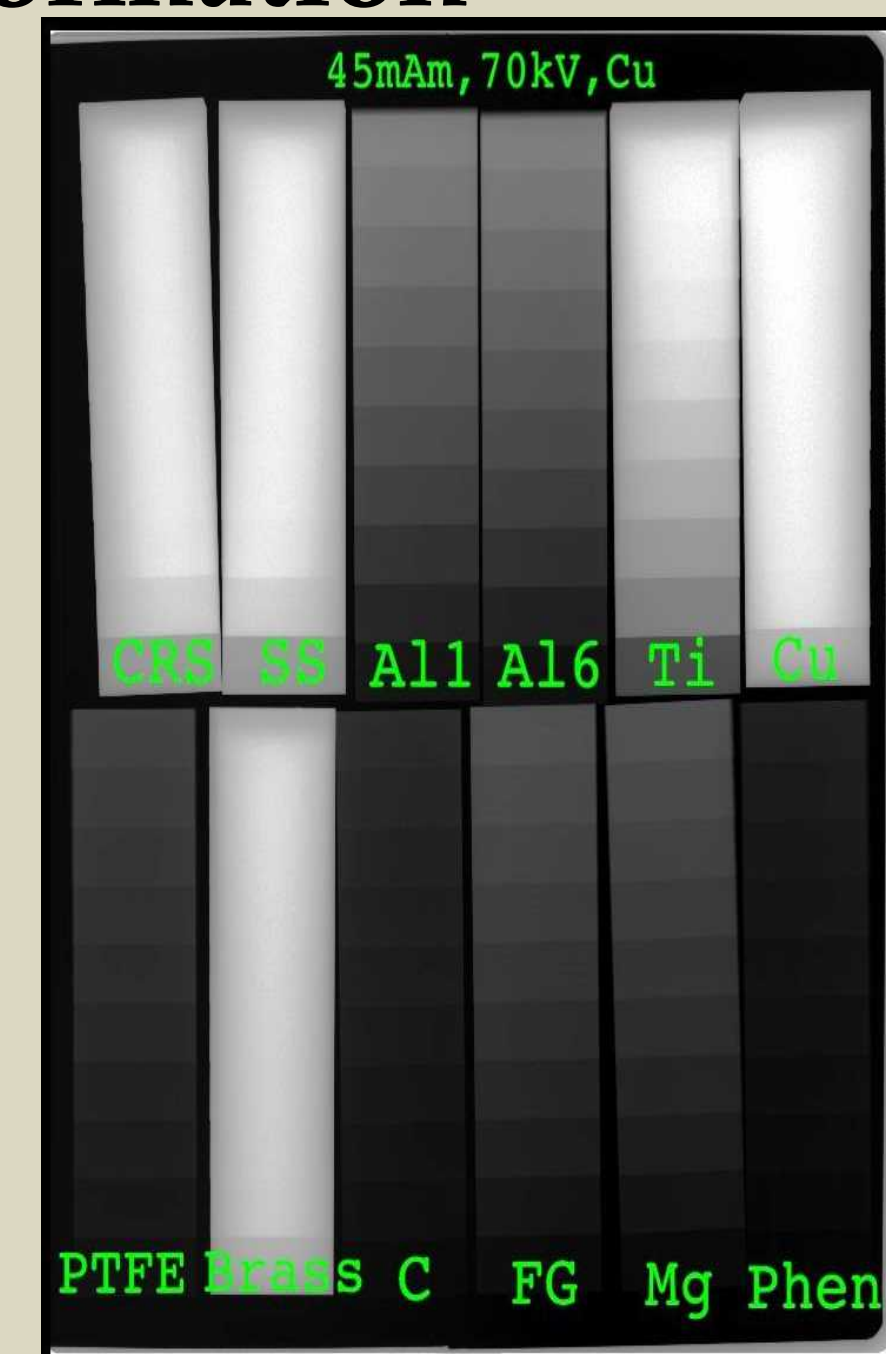
Example of a radiographic image with step wedges.
