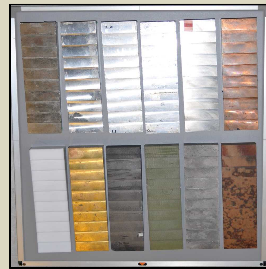
Left- Step-wedge have steps at 0.1 in intervals Right- Step-wedges as exposed on cassette
