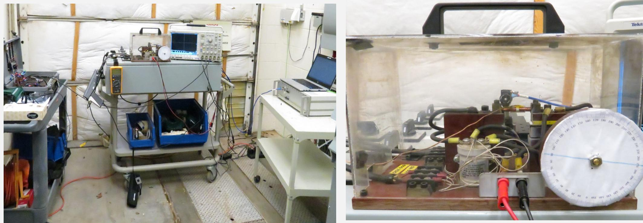
The S2000 Ocean Optics Spectrometer is coupled to a CCSA2 cosine corrected detector using a fiber optimized for high transmission efficiency in the UV-VIS wavelengths. The detector is positioned to collect signals from the electric discharge of the plasma.
