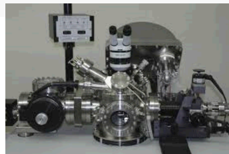
X-ray Photoelectron Spectroscopy (XPS): Detect oxidation state and chemical composition of product
