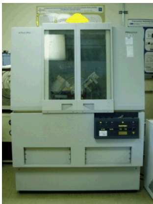
Powder X-ray Diffraction (PXRD): phase identification, degree of crystallinity
