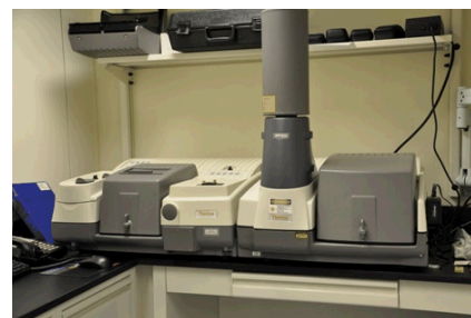
Fourier Transform Infrared Spectroscopy (FTIR): Vibrational modes to detect functional groups
