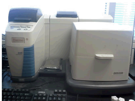
Raman Spectroscopy: Vibrational modes to detect symmetry
