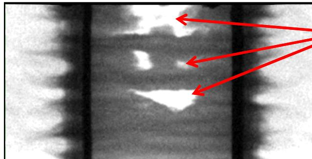
Time-integrated self-emission from liner implosion at 6151 eV; missing in shots with axial field
