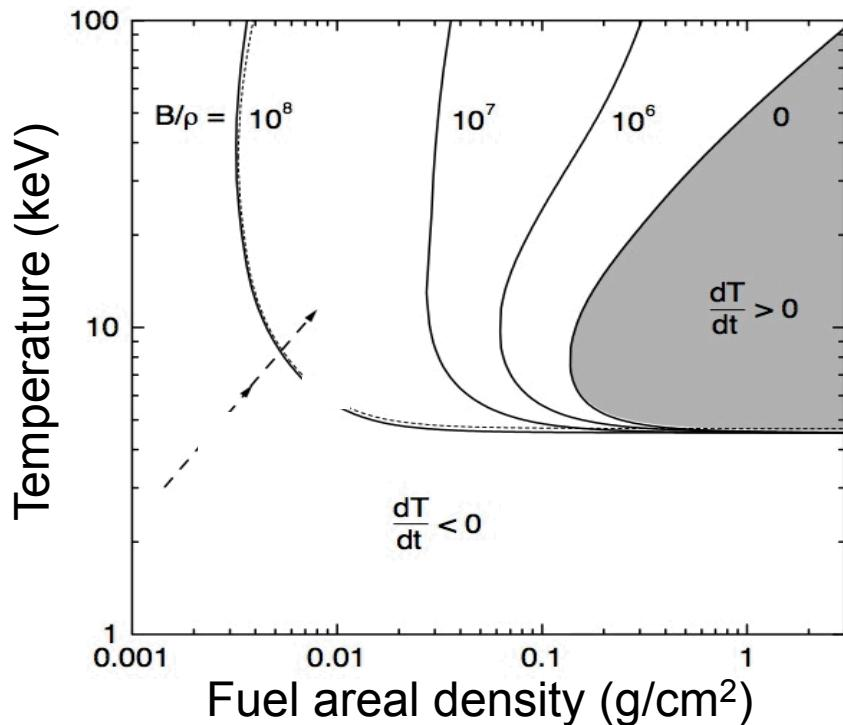
The  $\rho r$  needed for ignition can be significantly reduced by the presence of a strong magnetic field largely through inhibiting electron conduction
