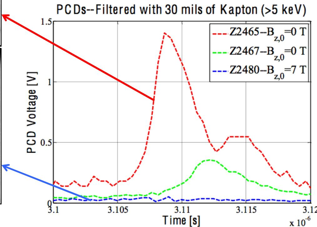
If magnetic flux roughly conserved the additional magnetic pressure from the axial field will suppress micro-pinching—this is indirect evidence for flux compression 22
