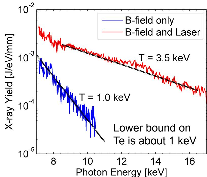
The measured electron temperature is close to the ion temperature obtained from neutron time-of-flight data; x-ray emission yields are consistent with fuel  $\rho \sim 0.4$  g/cm<sup>3</sup>
