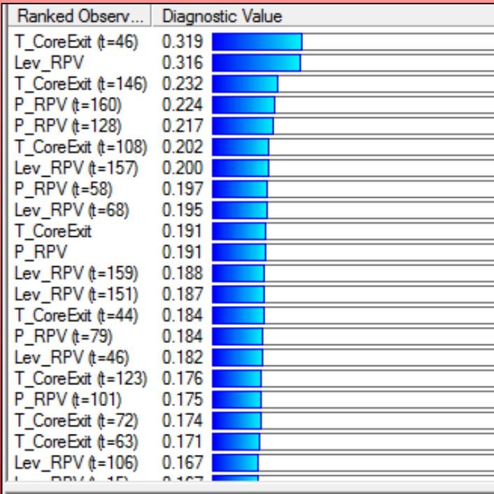
Suggested checks: Core exit temp (t46), RPV level(t0)
