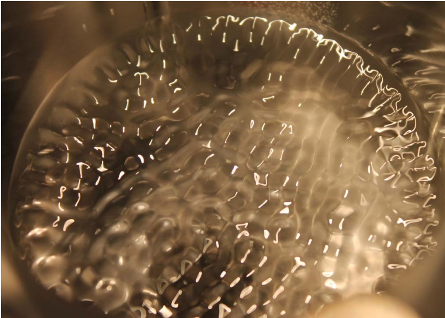
View of Faraday waves from above a vibrating free surface at: 80 Hz, 5 g, 76 mm dia, 25 mm depth, 20 cSt PDMS silicone oil
