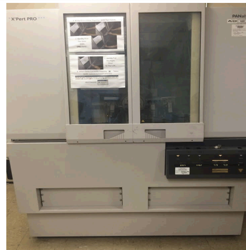
PXRD: instrument that characterizes the crystallization of a product
