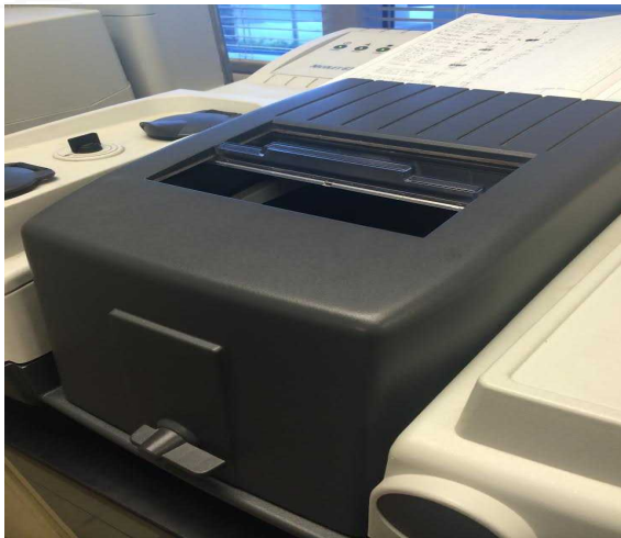
FT-IR: instrument that characterizes the functional groups of a product
