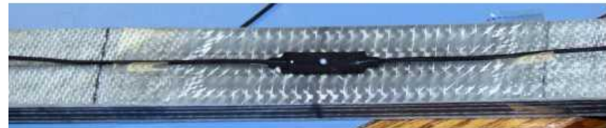
Figure 5 – Test specimen with a mounted MOI standard-package FBG sensor.
