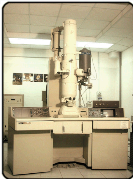
Transmission Electron Microscopy (TEM): characterizes crystallographic shapes and size
