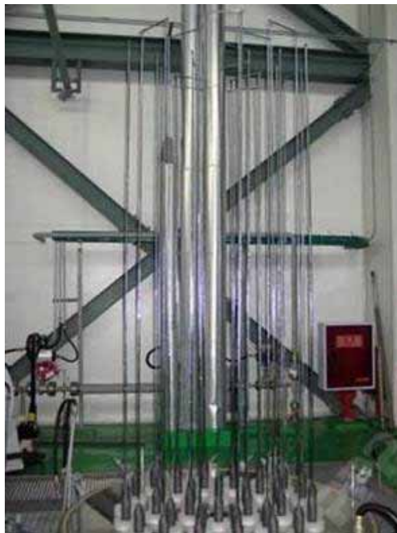
Before polysilicon growth – slim rods
