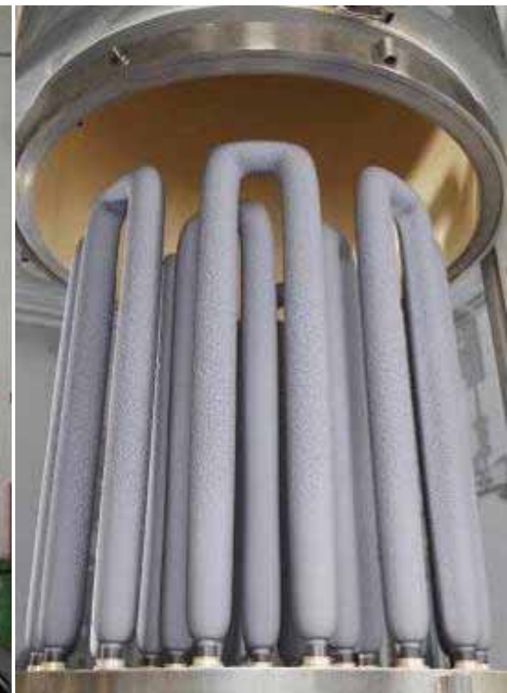
As grown polysilicon rods after a reactor run
