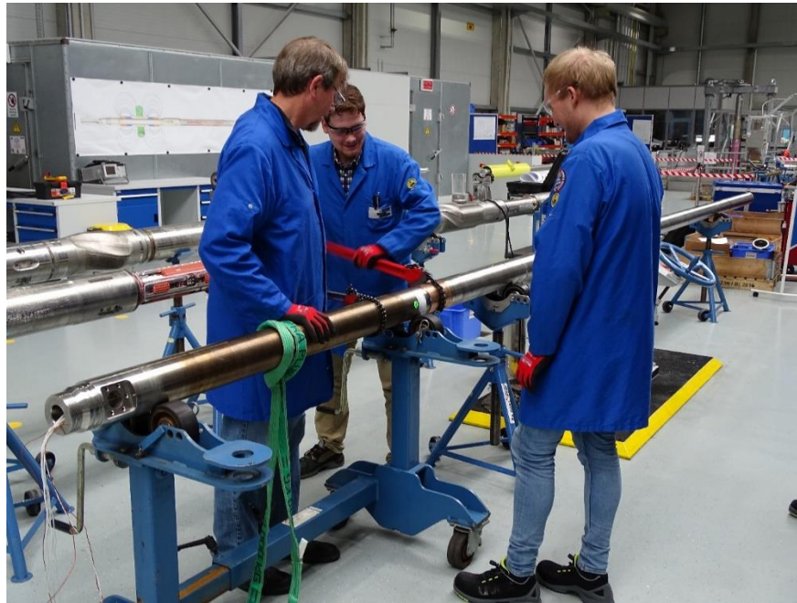
Figure 24 Assembly of the probe comprising Dewar flask, water container and Zeolite reservoir
