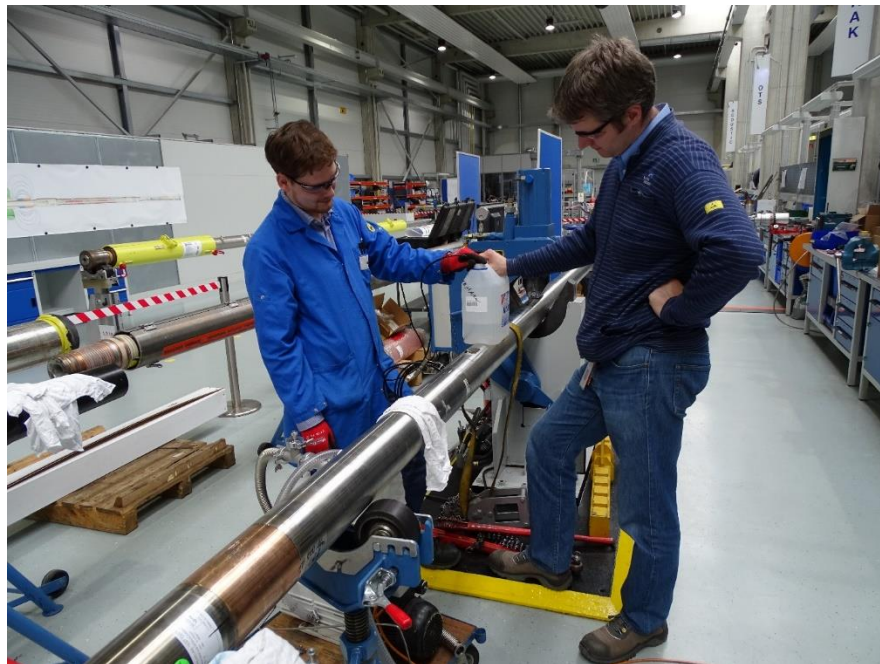
Figure 25 Preparation of the high temperature test of the active cooling system by filling 2.7 l water into the water tank
