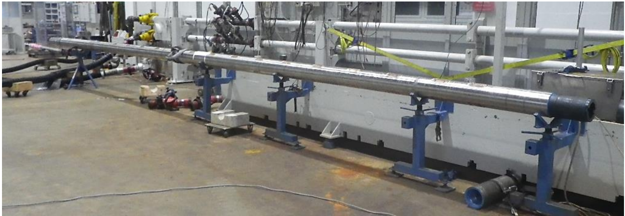
Figure 20 Low temperature flow loop testing of the assembly prior to shipment for field testing
