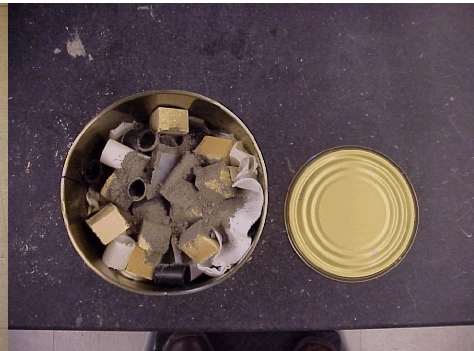
METALS: Steel Conduit, Copper Tubing, Can & Lid   PAPER, CLOTH, WOOD: Wood, Rags   PLASTICS: Polyethylene Pipe, Polyethylene Bottle, Polyvinylchloride Pipe, Gloves   SORBENTS: Portland Cement, Oilsorb
