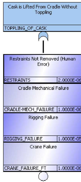
Figure 10-20. Fault tree 5.1, cask is lifted from cradle without toppling.
