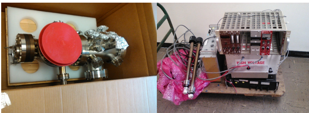
Figure 1. The Mott polarimeter vacuum chamber (left) and control electronics (right) as delivered from Jlab to Cornell University.
