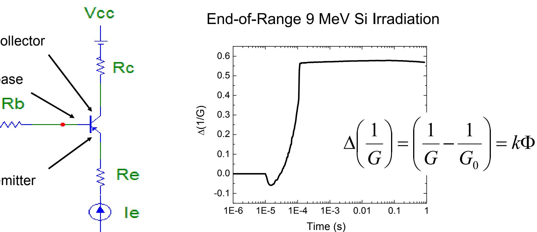
All devices operated at fixed emitter current of 0.22 mA, with a  $V_{BC}$  of 4 V
