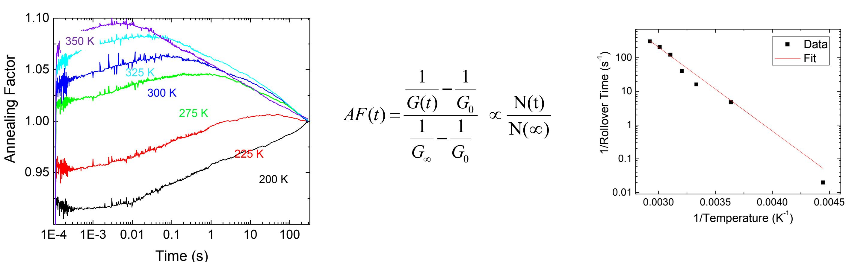
Observe a dramatic temperature dependence, plotting 1/roll-over time we find an Arrhenius behavior with a 0.5 eV activation energy
