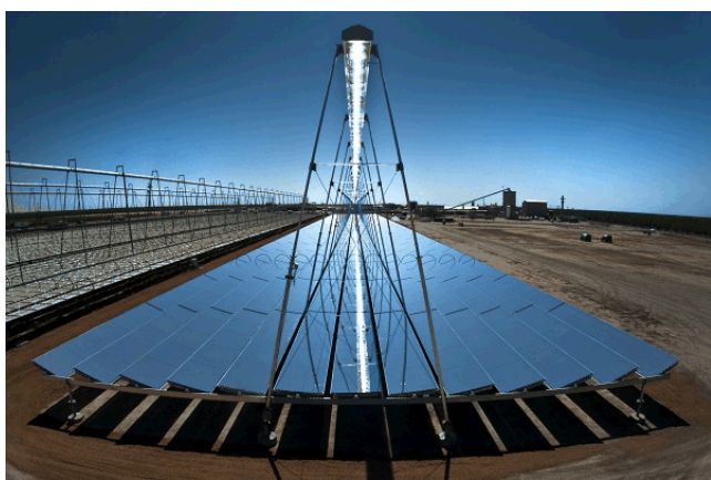
Figure 1. Configurations for Concentrated Solar Power applications. 1 From top left clockwise, a) parabolic trough, b) solar power tower, and c) linear Fresnel lens system.
