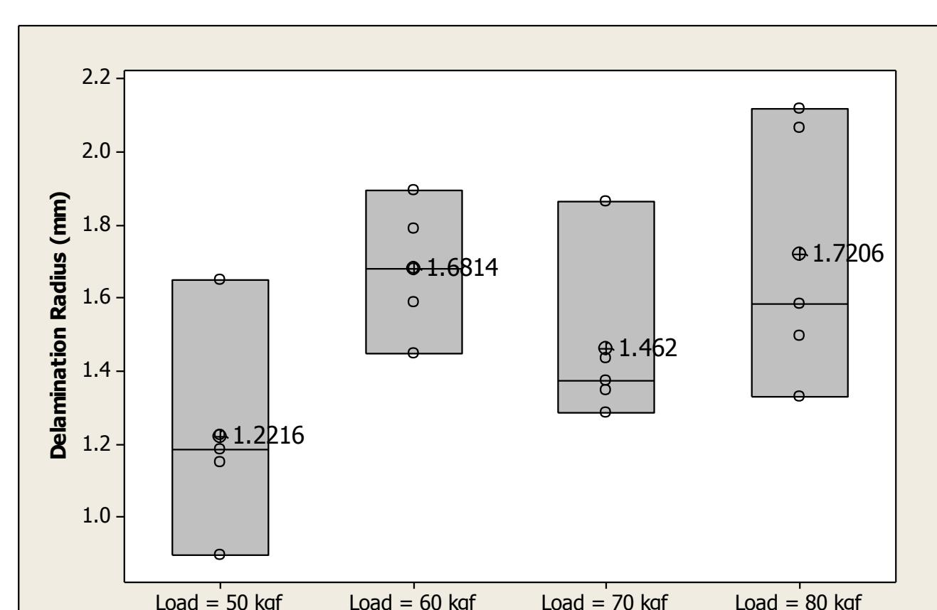
In general, delamination size increases with load.
