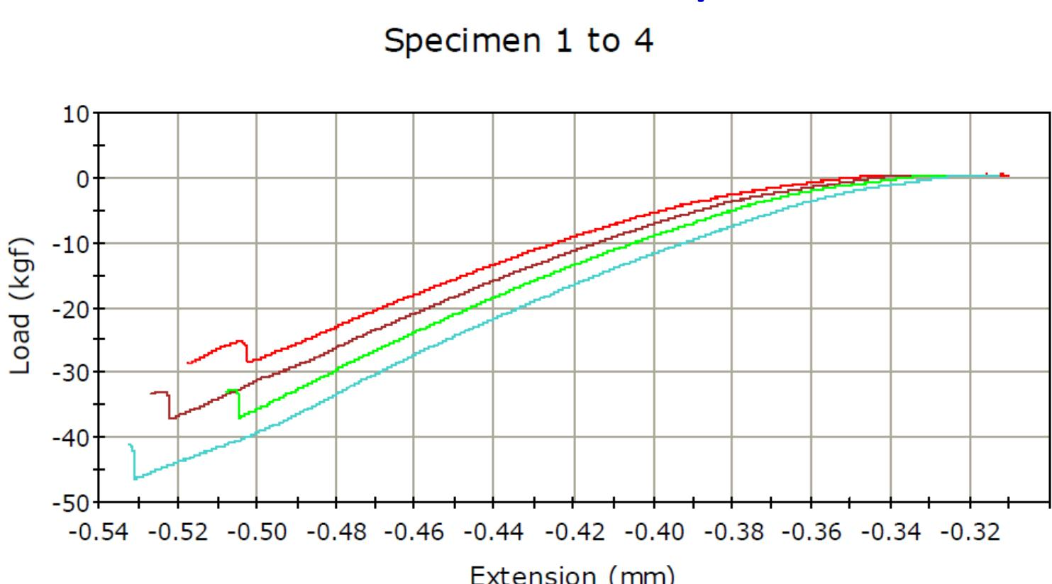
When delamination occurs, there is a small and sudden drop in load. The sample is then unloaded and moved to perform the next indent.
