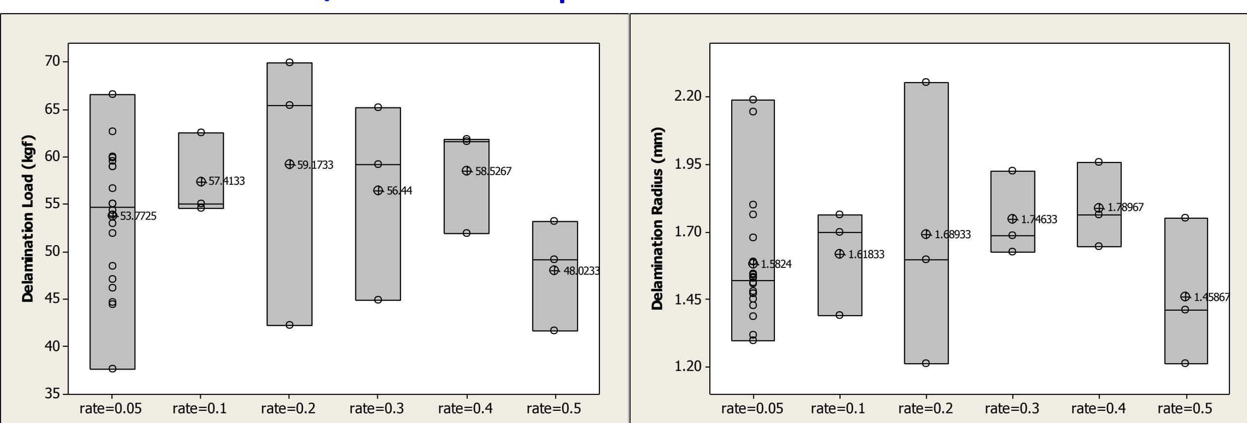
Based on these data, indenter speed does not appear to have an effect on delamination.
