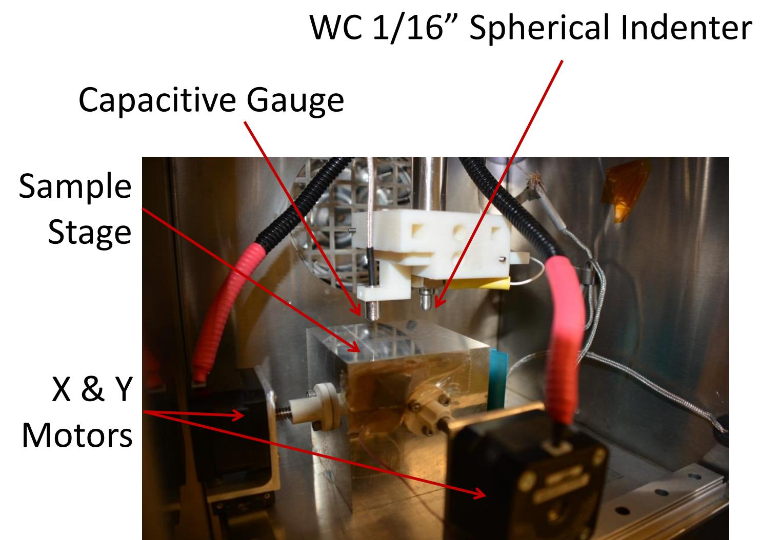
Indentations were performed with an Instron 5565. The indenter was attached to a load cell that was bolted to the bottom of the crosshead. A motor moved the crosshead down at a rate of 0.05 mm/min. An attached computer recorded the indenter load and crosshead displacement every 2 ms.
