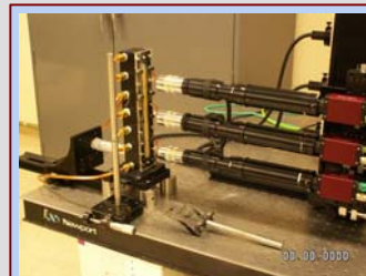
The bubble size testing apparatus. Water flows through the tubes to maintain the column at a reasonably constant temperature.
