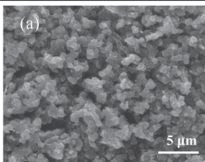
Figure 2. SEM Image of nanoporous carbon.
