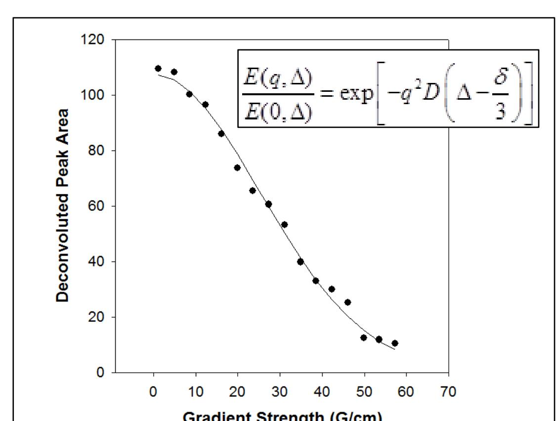
Figure 6. A decay of signal intensity from a diffusion experiment, fit to the Stejskal-Tanner equation
