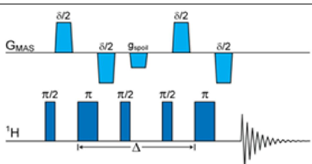
Figure 3. PFG stimulated echo with dipolar gradients and spoil gradient for <sup>1</sup>H-detected diffusion measurements.  $G_{MAS}$  indicates the gradient is applied at the magic angle.
