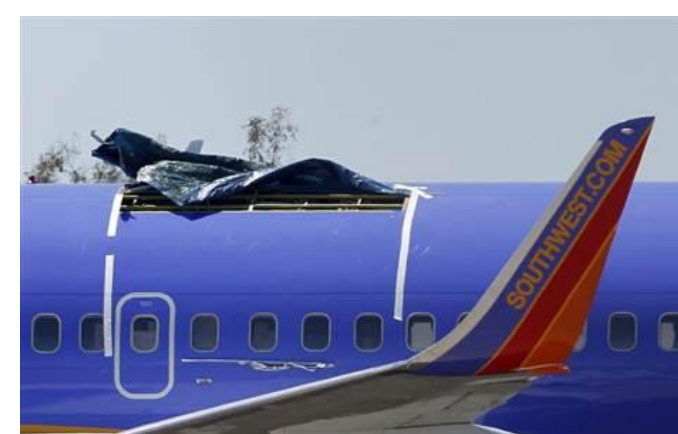
Roof failure of Boeing 737 aircraft due to fatigue cracks. From imechanica.org
