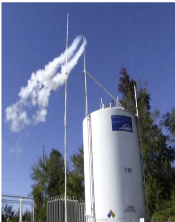
Fig. 6 – Deployment of the prototype Cold Hydrogen Plume Analyzer. During LH 2 venting through a 9.5 m (31.5 ft) stack.
