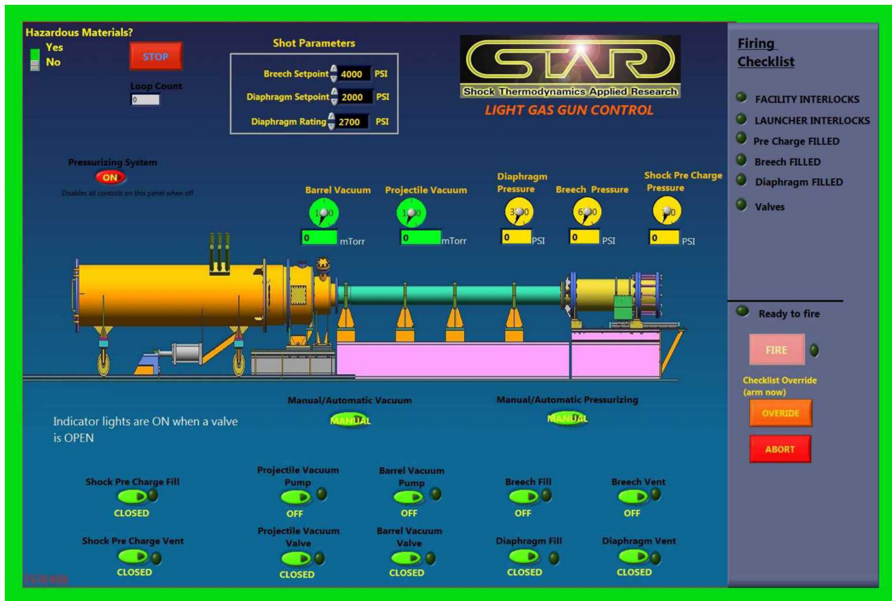
Figure 7. Front Panel User Interface for IVG Gun Operations
