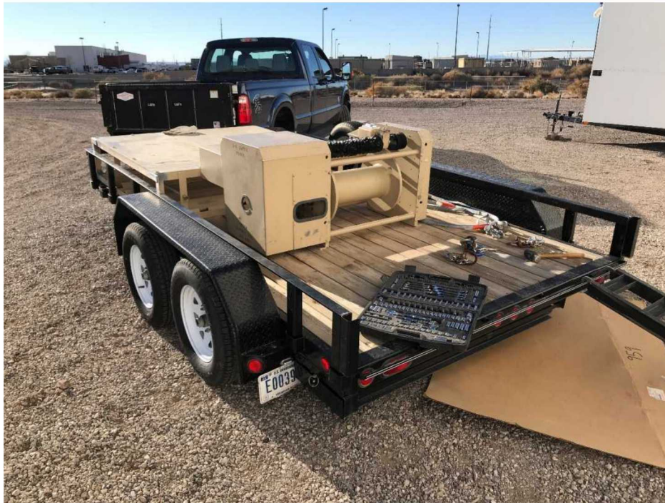
Trailer was reoutfitted with an old helium rack to add the capability of transporting helium cylinders. Winch was mounted to the frame of the trailer and 4" U-channel was added to further secure the winch to the frame.
