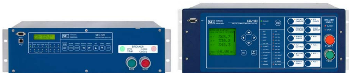
Figure 1 – Photos of SEL phasor measurement units (PMUs)
