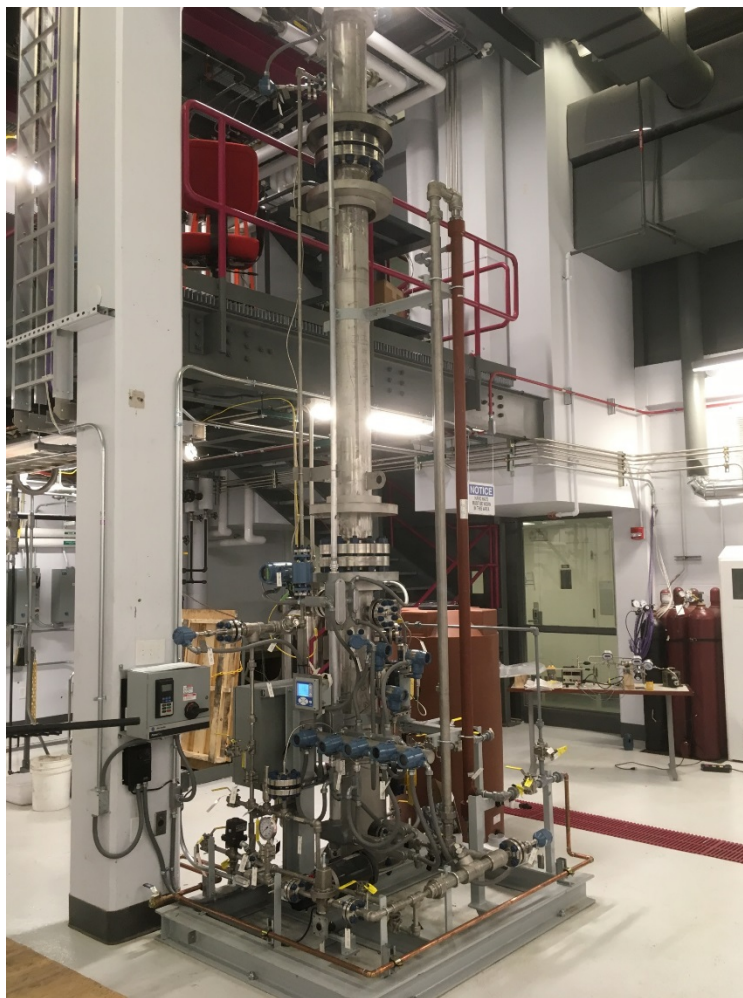
Figure 11. DCC scrubbing column installed at the pressurized oxy-combustion research facility at Washington University in St. Louis.
