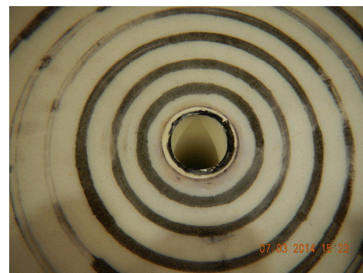
Small grain (#140 - #270) silica sand before and after draining.
