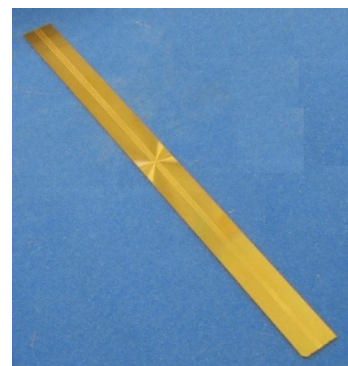
FIG. 4. Individual gold penumbral layer, 3 grooves scribed along the length.
