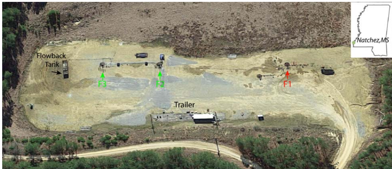
Figure 9. Areal view of the Detailed Area of Study at Cranfield, Mississippi (Lon: -91.141^\circ , Lat: 31.564^\circ ), which consists of an injector (F1) and two monitoring wells (F2 and F3). During leak experiments, F3 was used as a “leaky” well. Locations of the flowback tank and trailer area are also labeled.
