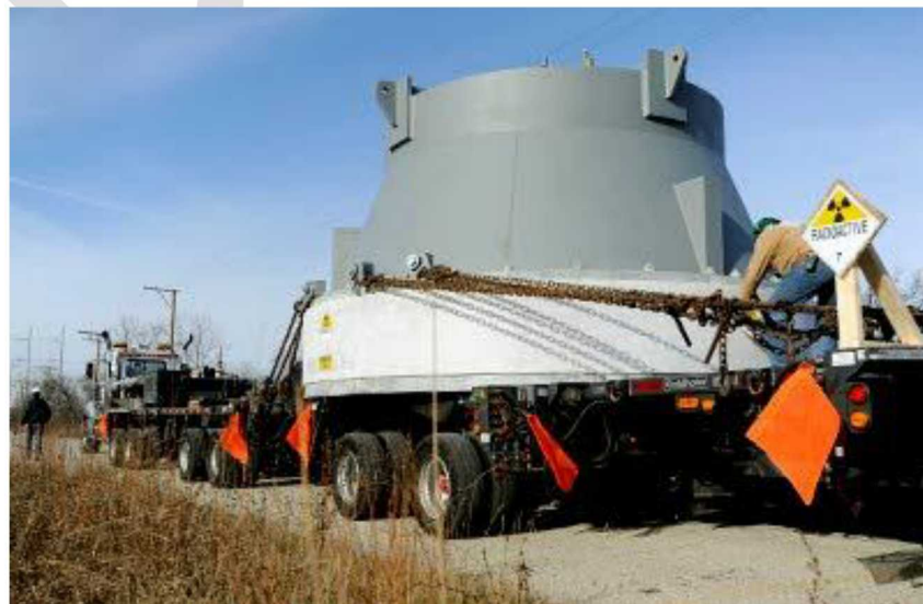
Figure 4-16. Zion Reactor Head on Heavy Haul Truck Transporter
