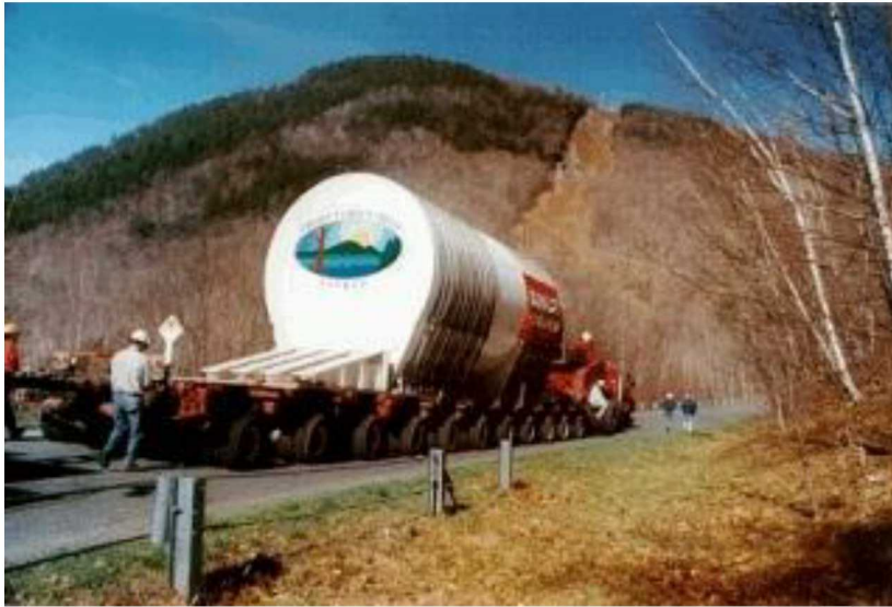
Figure 4-7. Yankee Rowe Reactor Pressure Vessel on Heavy Haul Truck (Yankee Rowe 2012)
