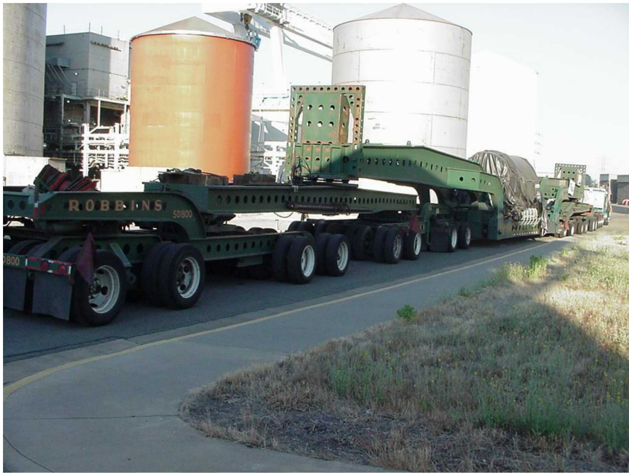
Figure 4-6. MP187 Cask Transported by Heavy Haul Truck
