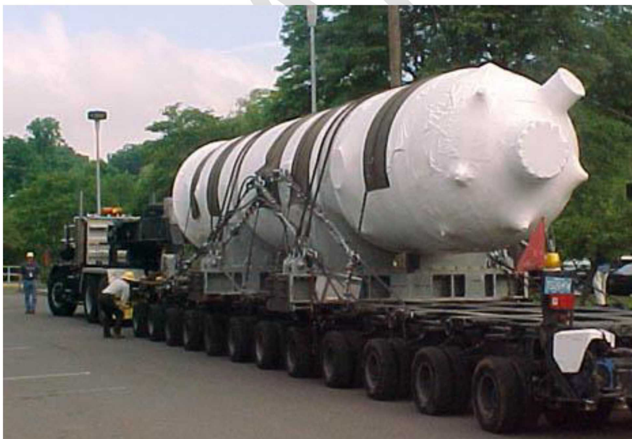
Figure 4-13. Connecticut Yankee Pressurizer on Heavy Haul Truck Transporter (Connecticut Yankee 2012b)
