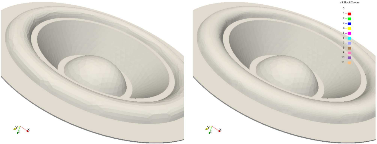
Figure 3.5: Example of UMR with geometry from mesh-based geometry: two levels of uniformly refined meshes.
