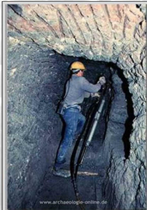
Headwork with jack-hammer in old-drifts in the salt mine Dürnberg (A)
