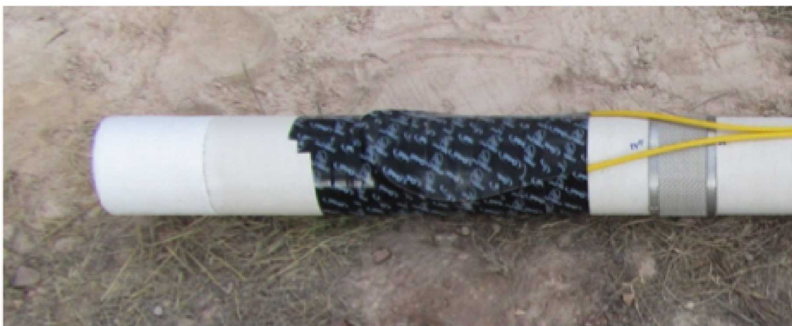
Figure 4.6. Fiber optic cable (distributed sensing) was deployed on the exterior of the casing. To avoid unnecessary splices in the cable, the cable was looped at the bottom of each monitoring borehole and secured with duct tape. This also provided twice as many DAS measurements in the boreholes.
