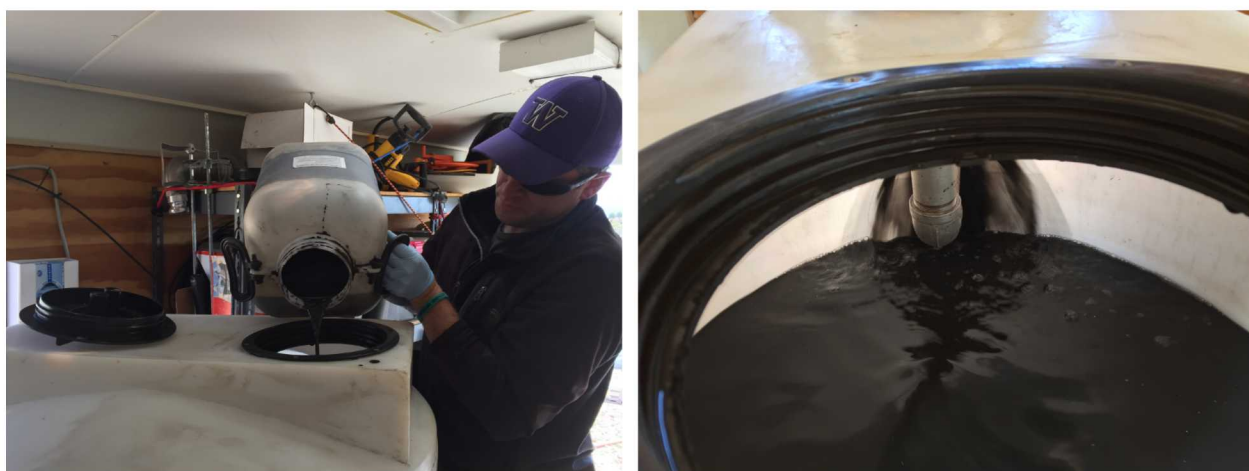
Figure 13.1. Zero-valent iron and diethionite reductant solution (right) applied to the mixing tank (right) prior to injection into the stimulated fracture zone.
