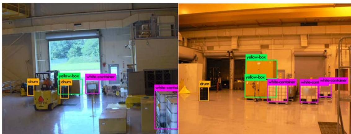
Fig. 5 Example images of object detection by the YOLO v3 model. The images show the operation of the BNL Waste Management facility. Three defined classes of objects were detected with good accuracy.
