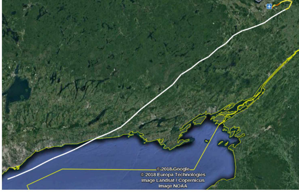
FIG. 2.1. Partial Trajectory of Flight A3A458 in which sampling begins mid-flight over Lake Erie and ends with landing in Ottawa. White segments are straight; Yellow segments are left turns; Orange segments are right turns.
