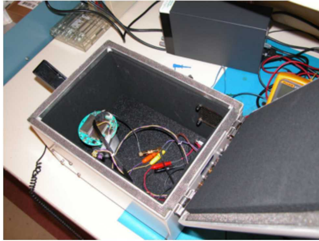
Figure A.14: 64-element SiPM array with a 26.0VDC bias voltage coupled to the CsI crystal inside the shield box.
