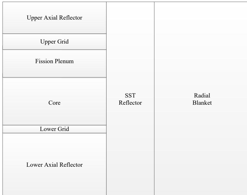
Fig. 4.17 Vertical Layout of EBR-II Run 163A
