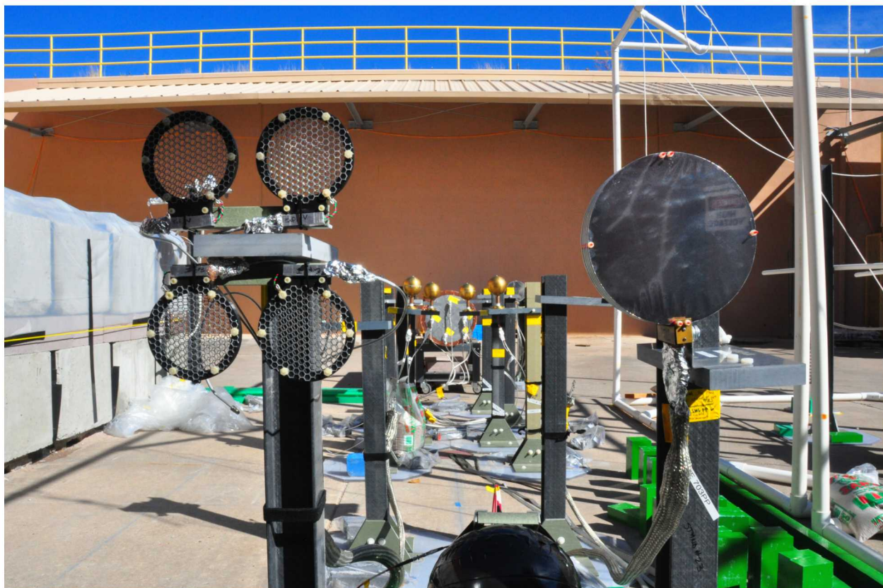
Figure 5: Photograph of the mesh conductivity sensors and the 703 pie pan sensor on their mounting stands.
