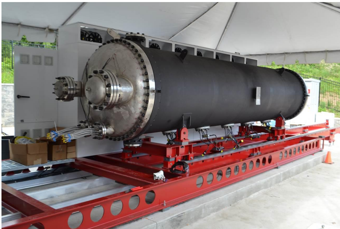
Figure 24 Fuel Cell Vessel Installed on Generator Module Frame
