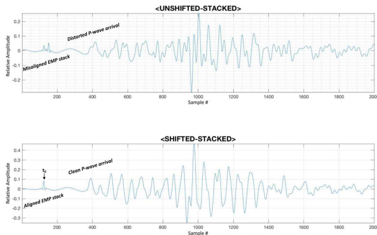
Figure 3-3. At top, stacked data trace from CBCD-4 showing results of stacking traces with timing errors. At bottom, same trace stack showing results of timing correction in which the aligned EMP peak is then assigned as t_0 for the stacked shot record.
