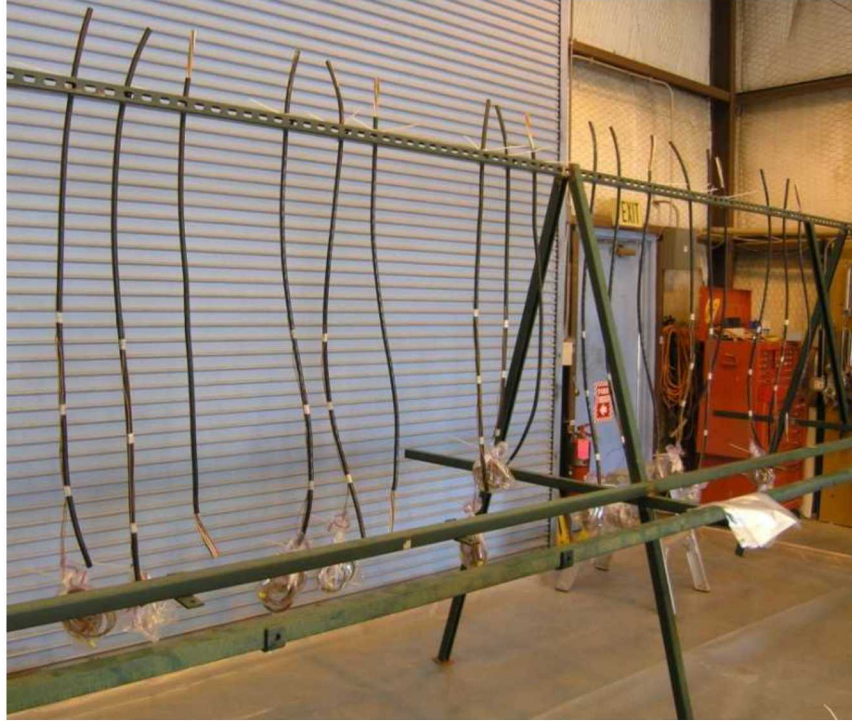
Figure 7. Welded A-frame used to suspend single lengths of cable for the coating process
