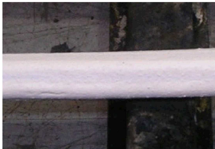
Figure 4. Fully cured Vimasco 3i on a cable sample
