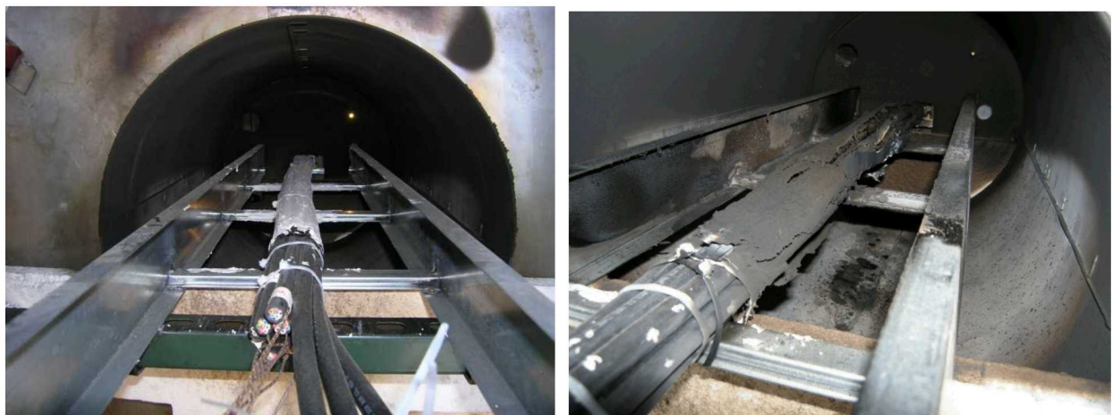
Figure 33. Before-and-after photos of the cable bundle separation behavior
