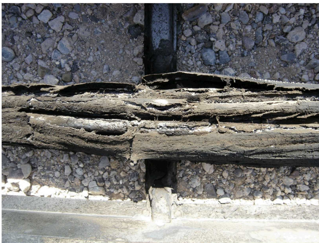
Figure 34. Close-up photo of separated cable bundle
