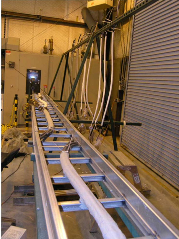
Figure 10. The curing of bundled and single lengths of cables.
