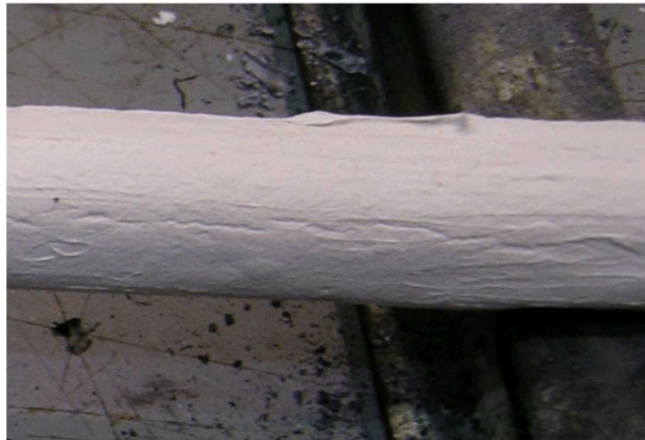
Figure 3. Fully cured Flamemastic F-77 on a cable sample
