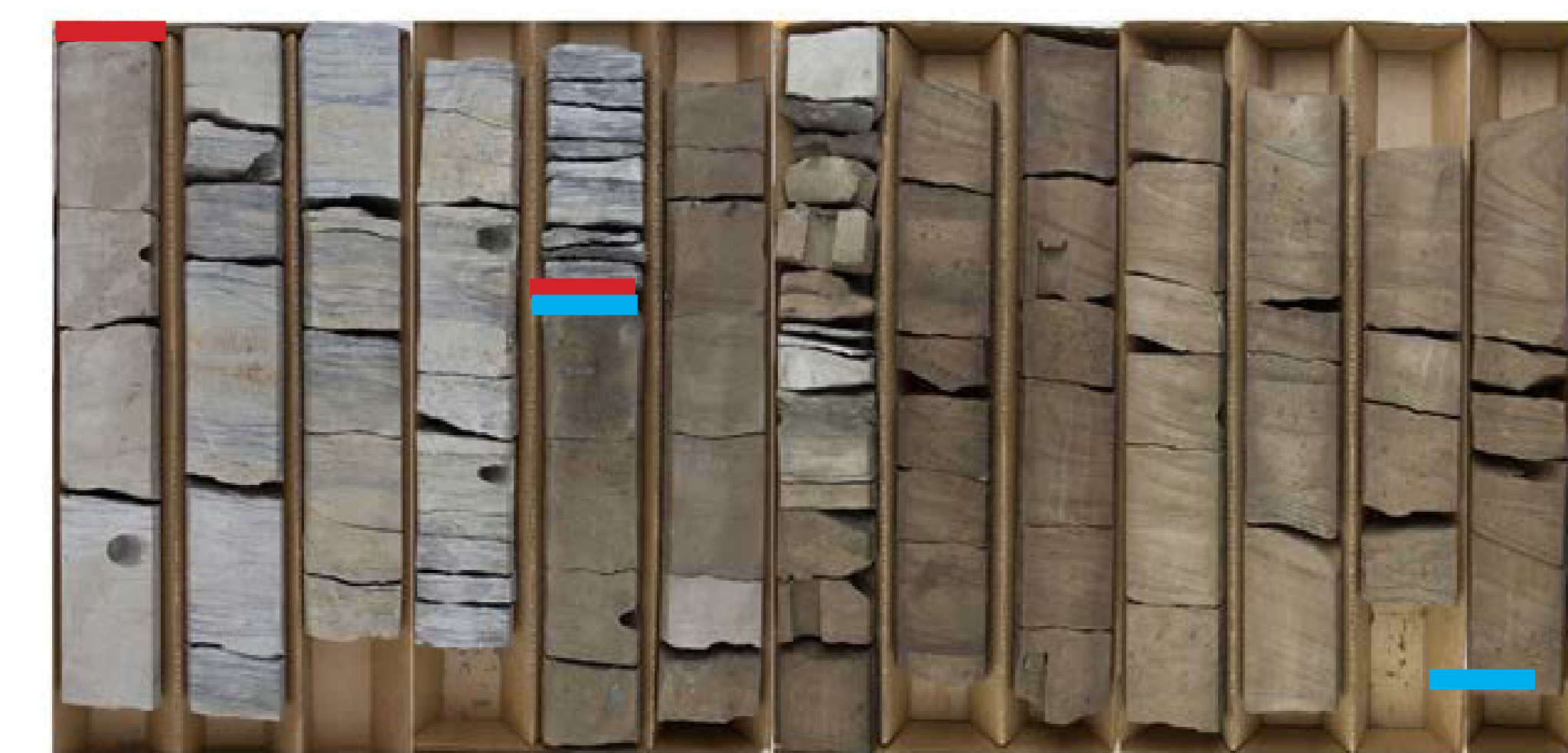
Figure 3: This picture shows the Montgomery B-34 core. It begins in the top left corner and continues down to the bottom right corner. The section bounded by the red lines includes the lenticular- and wavy-bedded sandstone. The section bounded by the blue lines includes the ripple- and cross-bedded sandstone.
