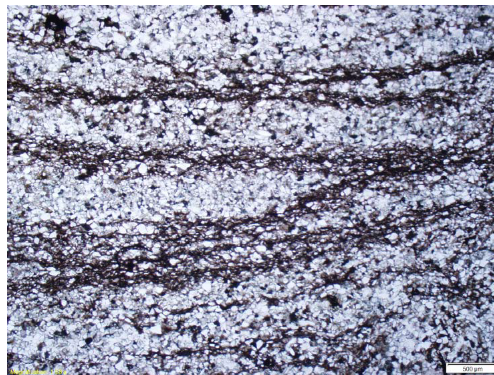
Figures 10&11: These photomicrographs show the composition at 2583.5 ft. Each picture is showing the same depth at a different scale. Clay interbeds can be seen cutting across the slide; they are more numerous than the wavy-bedded facies.
