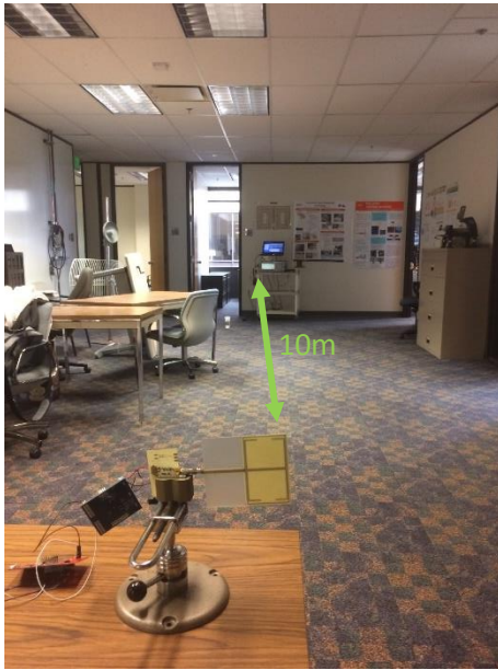
Figure 3 Sensor tag transmitting data over 10 m
