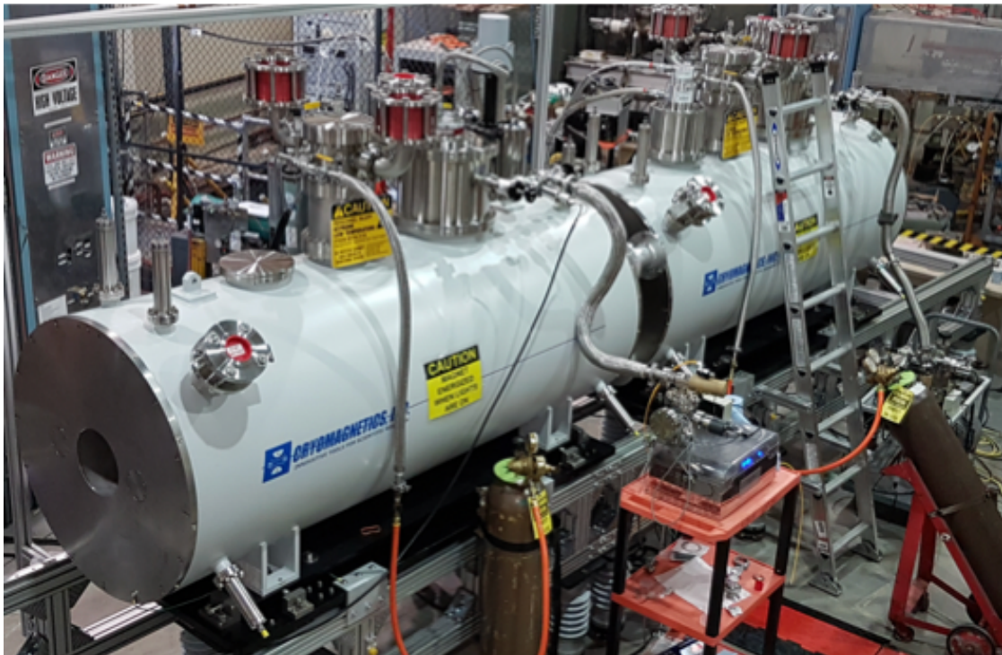
Figure 6. The reinforced 5 T superconducting solenoid magnets for the Extended EBIS Upgrade.
