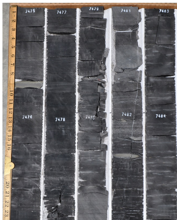
Figure 9: MIP-3H core photographs, from 7,475 to 7,485 ft.
