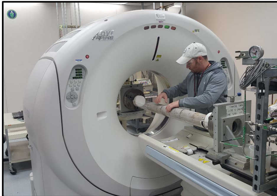
Figure 18: Toshiba® Aquilion™ Multislice Helical Computed Tomography Scanner at the NETL used for core analysis.
