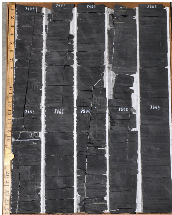
Figure 11: MIP-3H core photographs, from 7,495 to 7,505 ft.
