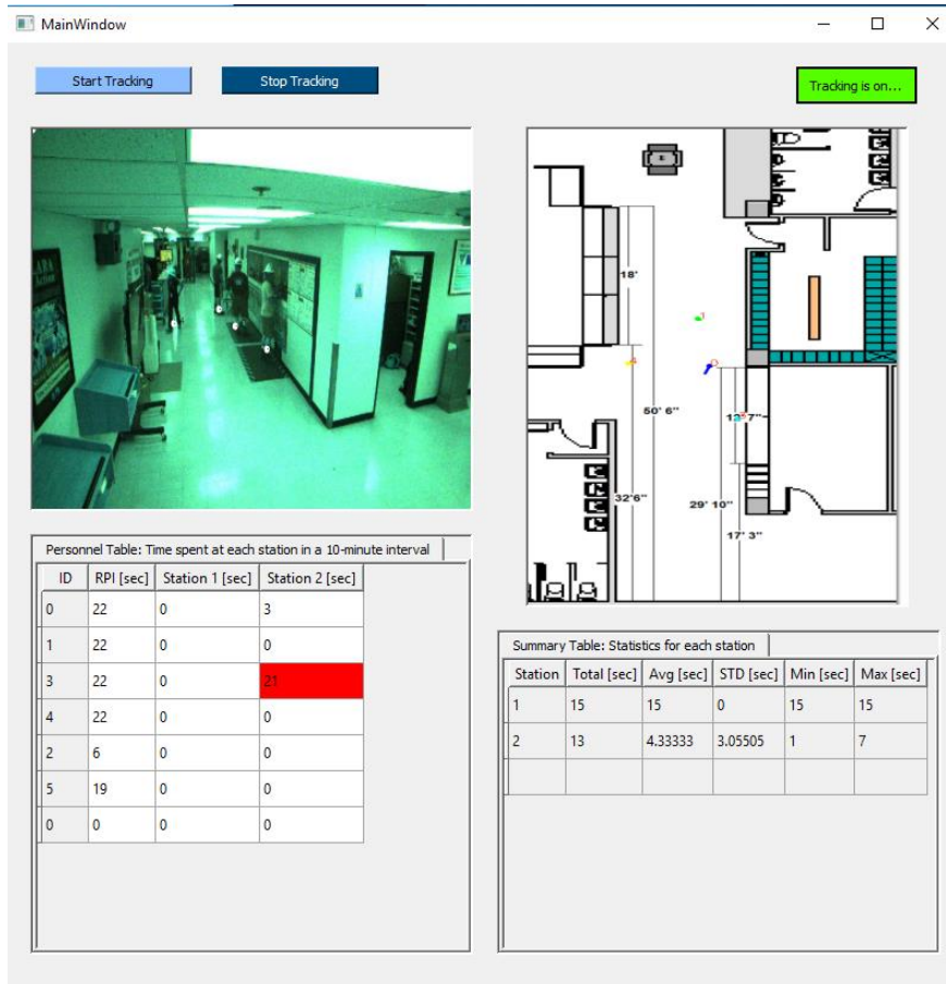
Figure 62 Real-time monitoring and statistics output (Red cell indicates the time worker spent in the station exceeded the alert limits)
