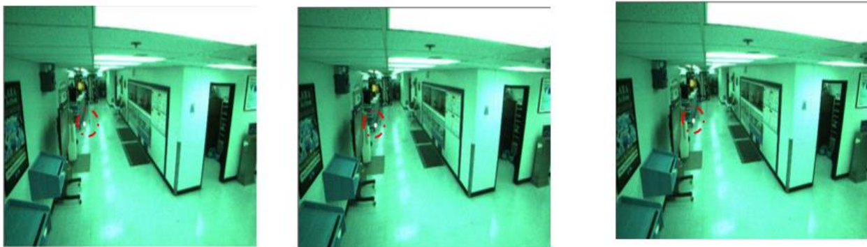
Figure 21. False detection due to reflective objects (red circle the false detection, the algorithm detected one worker in the video, whereas there is no worker)
