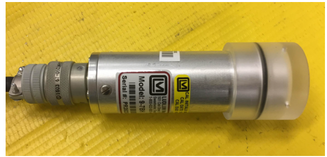
Fig. 2. Radiation detection instrumentation Ludlum Model 9-7.
