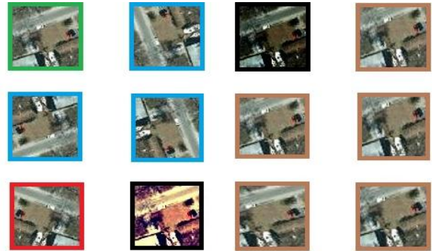
Fig 2. A visual guide to the data augmentation strategies employed for the creation of our custom data set. The Green image represents the original image. Blue represents the Rotated images. Red is the Mirrored image. Black are the images after Contrast Adjustment, and Brown are Randomly Cropped images.
